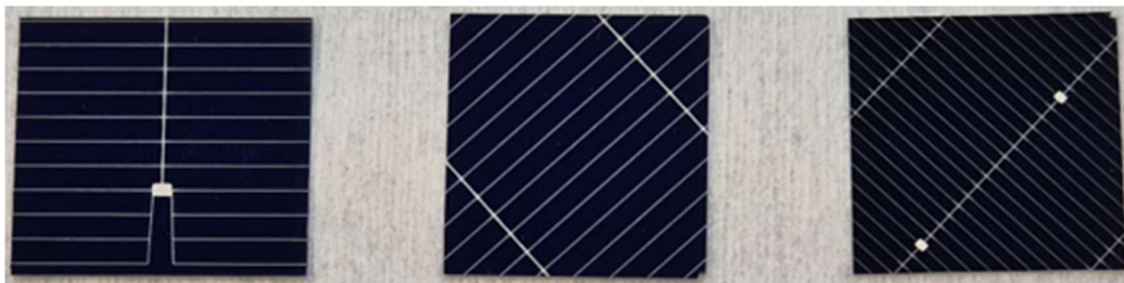
Figure 3: Left pane: Laser-scribed and mechanically cleaved SHJ solar cell. Middle pane: Mechanically cleaved SHJ solar cell using a diamond scribe. Right pane: Mechanically cleaved TOPCon solar cell using a diamond scribe. The cell size is about 2 \times 2 \text{ cm}^2 .
